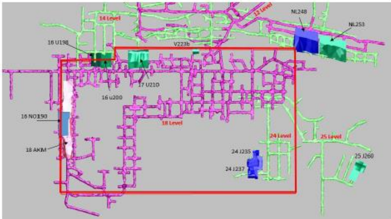
Fig. 4: Plan view of Nifty underground development, showing planned stopes (coloured shapes) for FY2019 and the checkerboard (CCB) outline in red.
