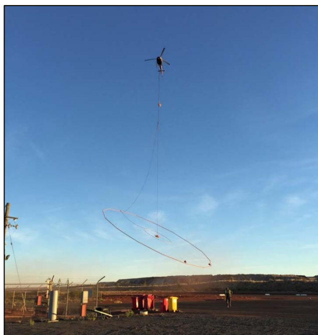
PHOTO 2: VTEM SYSTEM TAKING OFF FROM NIFTY AIRPORT TO START SURVEY THROUGH THE MAROOCHYDORE PROJECT
