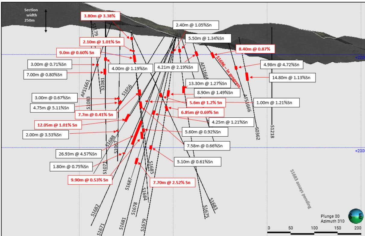
Figure 2: Section (250m width) looking north showing new (red text), and previously reported and historic (black text) Sn intersections. Intersections are shown as downhole widths.
